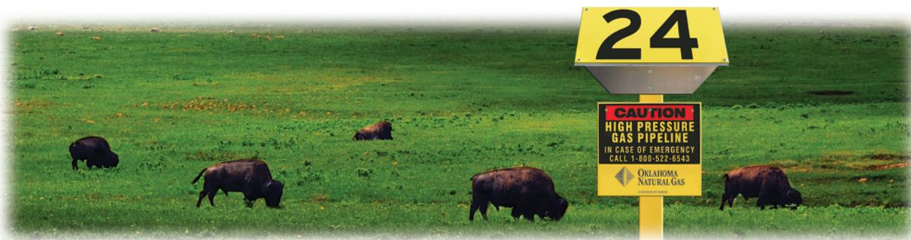
A pipeline right of way is a strip of land over and around buried pipelines that allows them to be permanently located on public and/or private land to provide natural gas service. Rights of way should be kept clear of obstructions to enable Oklahoma Natural Gas employees to safely operate, patrol, inspect, maintain and repair natural gas pipelines.
